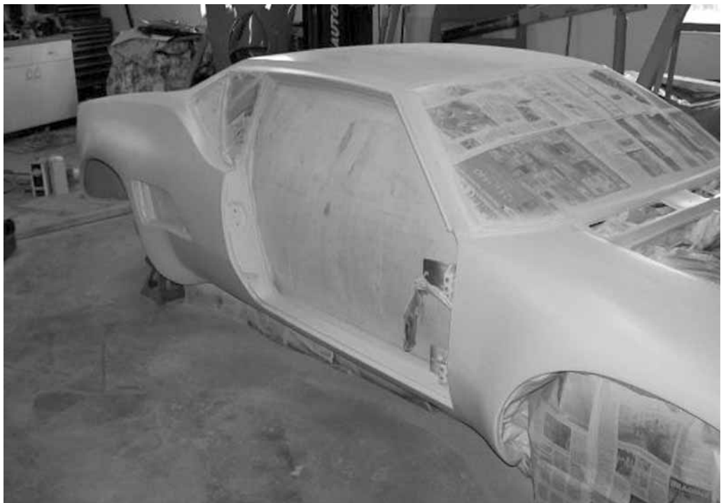
With the bodywork complete, several coats of primer were laid down
