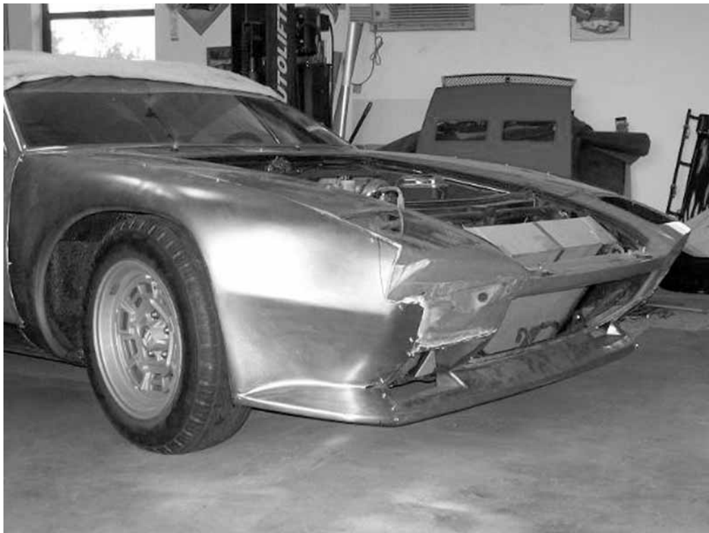
The De Tomaso fender and the Hall Pantera front end came together perfectly after some minor tinning
