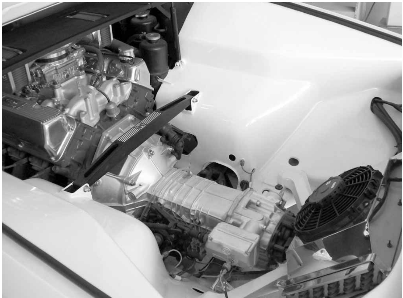
The engine bay was completely cleaned and painted the same as the exterior of the car. The engine was cleaned and the essential accessories replaced, but since the 1971 motor came from the factory with the desirable closed-chamber heads and a fairly aggressive cam, and had very low mileage, he decided it didn't need to become a part
